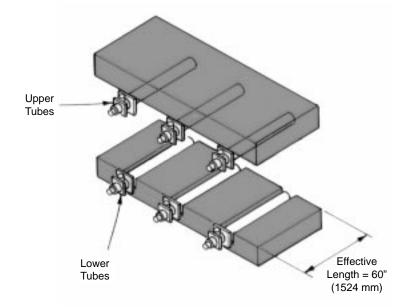
Upper tubes are free to radiate on three sides. Lower tubes are closely enclosed.
